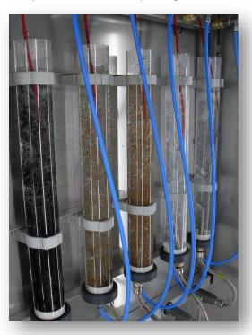
Each cylinder can run with its own day/night and temperature regime for testing several protocols at one run. We can also supply a "sophisticated" control system with logging to have more sight on the complete process.
