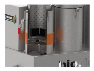
The BioRinse 5L can be modular configured, you can combine several washing stations with a centrifuge and multiple dryers and/or make any other possible combination. The complete system is controlled by a PLC system combined with an user friendly HMI.
