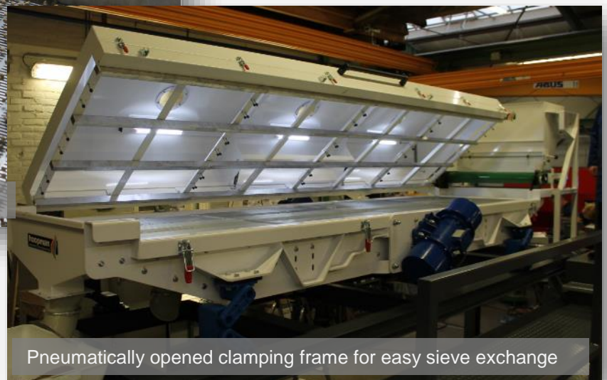
Accurate calibration due to vibration motors
