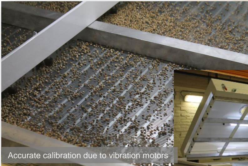
Accurate belt infeed system with fine setting
