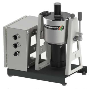
Fast, easy and complete discharge of the coated seed because there are no door-hinges, liquid distribution plate etc. Basic configuration with liquid disk in top cover part, with main disk on/off and speed regulation and setting of disposable syringes to quickly apply the slurry on the seed. Also powders can very easily be dosed onto the seeds. The 2 built-in mixing blades will mix the seeds easy and quickly for a good mixture of seeds and applied products.
