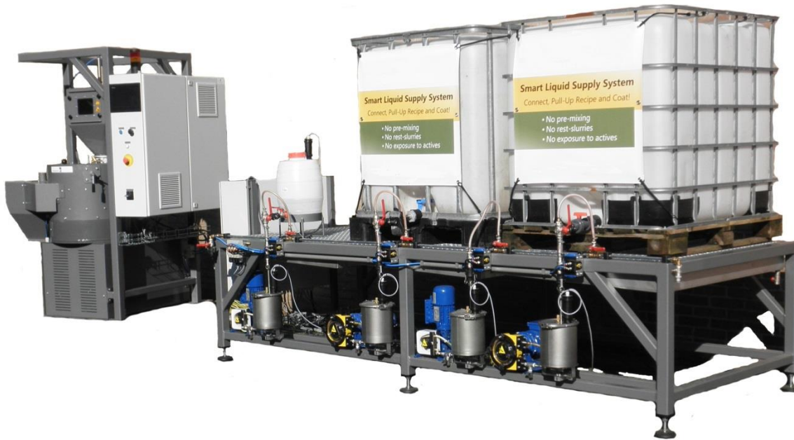
(Displayed version is 1x Basic unit + 2x IBC extension and 1x extra dosing system for water)
