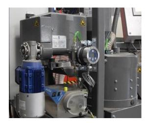
For fully automatic systems we also deliver bespoke weigh-out and feeding systems for the powders to be supplied. The powders will be pre weighed and put into the powder feeder for application. Ask us for more information about this bespoke systems.
