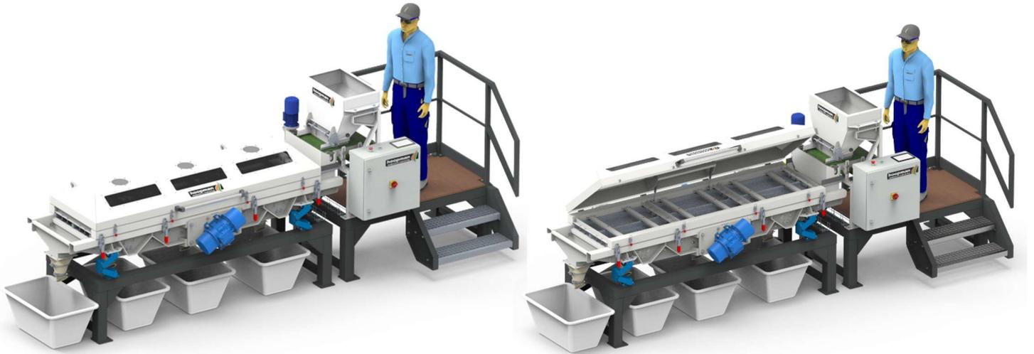
The sieve system is standard equipped with an inlet system, dust hood and control box to make it plug & play. 3 sieves of 600x800mm can be placed inside the frame to sort your product into 4 fractions.
