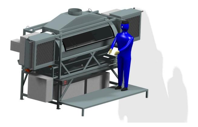
The heating can be done in several ways, the most simple way is to use Hot Water Heat Exchangers.
