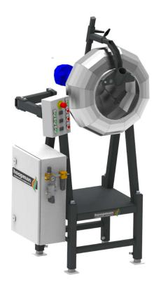
The pan coater is a machine for manual coating of small seed lots from 20-250gr. The pan coater is equipped with a specially segmented drum for optimal material movement and mixing during the process. For the PC-S we have 2 sizes pans available, the standard 600mm pan, and a smaller 340 mm pan. Due to the technical design it is possible to quickly change the pans by just one person.
