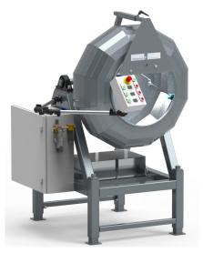
The pan coater is equipped with dust extraction from the back of the pan which makes the process better accessible and the operator is much less exposed to the often dusty process (also depends on materials used).
