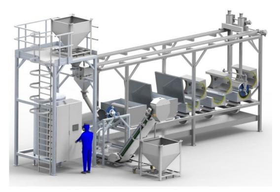
Just place a container full of seeds on top of the installation and place a collecting bin underneath the belt. Then press start and run completely automatic. The complete system has good accessibility for check during switch between several seed lots. This makes the unit easy to operate and easy to run.
