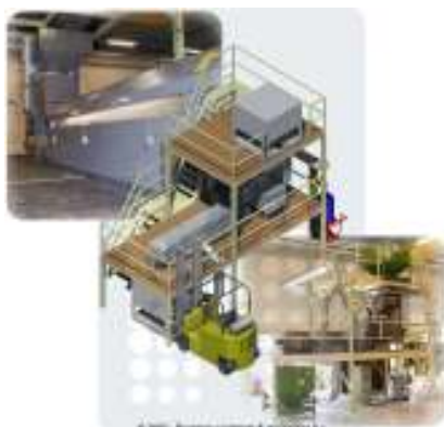
Rotary Fluid Bed Dryer connected to a HR600 (600 mm =15 ltr.) rotary coater
