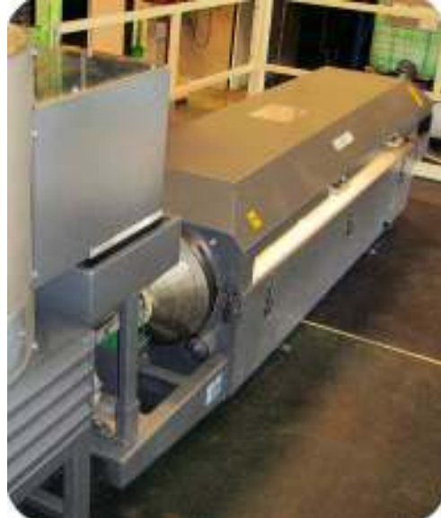
RFBD 400 connected to coating system
